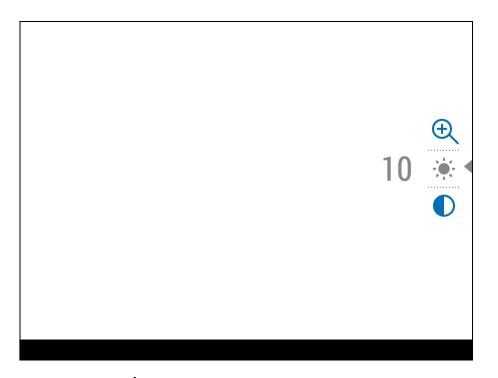
**Brightness**  $\dot{\Phi}$  - press the **UP (5)/DOWN (3)** buttons to change display brightness from 0 to 20.
