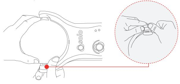
Fit the ASD adaptor by locating into both arms. Ensure that the fan symbol is located on the side of the unit where smoke is emitted. (LHS when unit is facing the user).
