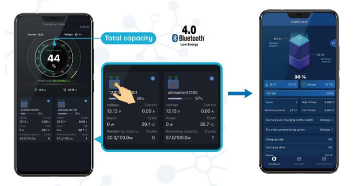
In single battery mode, click this button to switch any battery on each function page.
