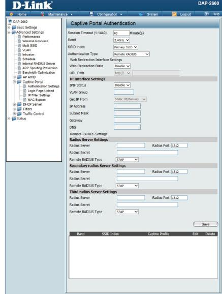
**IP Address:** Assign a static IP address that is within the IP address range of your network.
