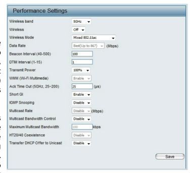
Transmit Power: This setting determines the power level of the wireless transmission. Transmitting power can be adjusted to eliminate overlapping of wireless area coverage between two access points where interference is a major concern. For example, if wireless coverage is intended for half of the area, then select 50% as the option. Use the drop-down menu to select 100%, 50%, 25%, or 12.5%.
