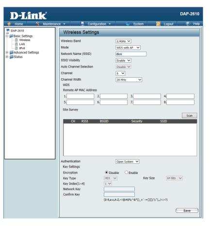
Remote AP MAC Address: Enter the MAC addresses of the APs on your network that will serve as bridges to wirelessly connect multiple networks.
