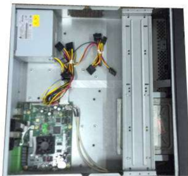
Figure 3-45 Put bracket back
