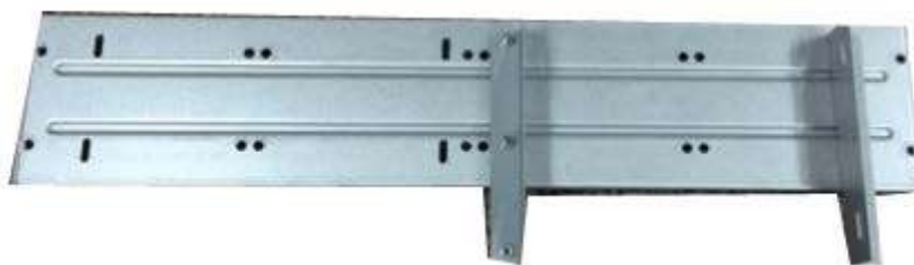
Figure 3-42 Install bracket (reverse side)
