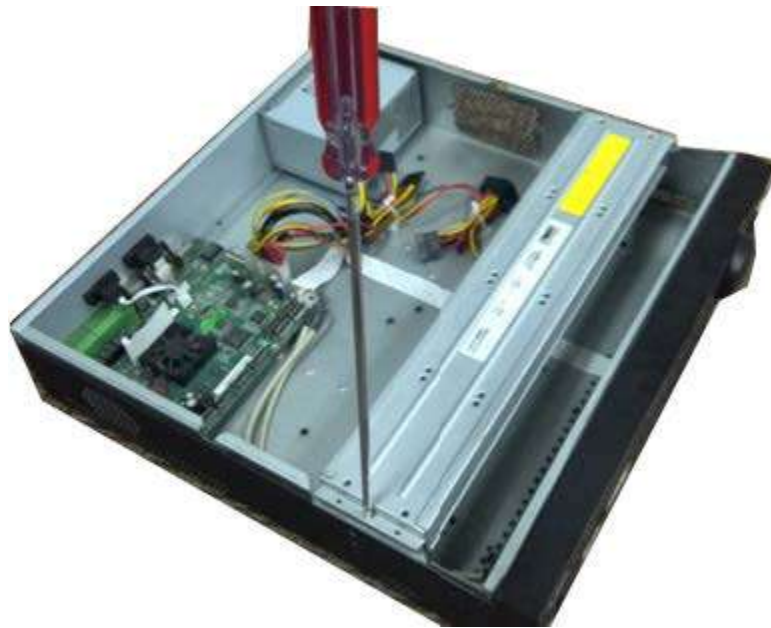
Figure 3-37 Open the top cover
