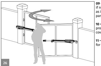
**09** • Test the door manually and if necessary readjust the micros, as indicated in the previous paragraphs.
