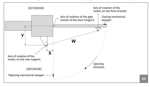
On the Illustrated diagrams below and on the next page, are the **dimensions for the installation** of the automated system.
