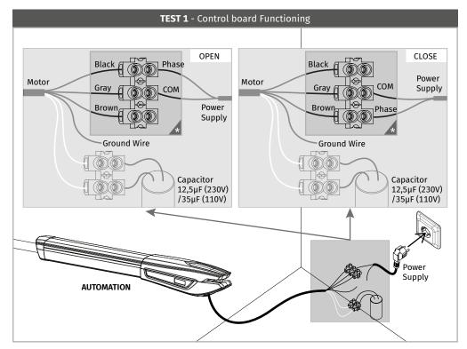
01 • Connect the 3 automation wires in the terminal.
