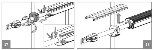
**02** • Loosen the 3 front screws, remove the cover and the profile cover.
