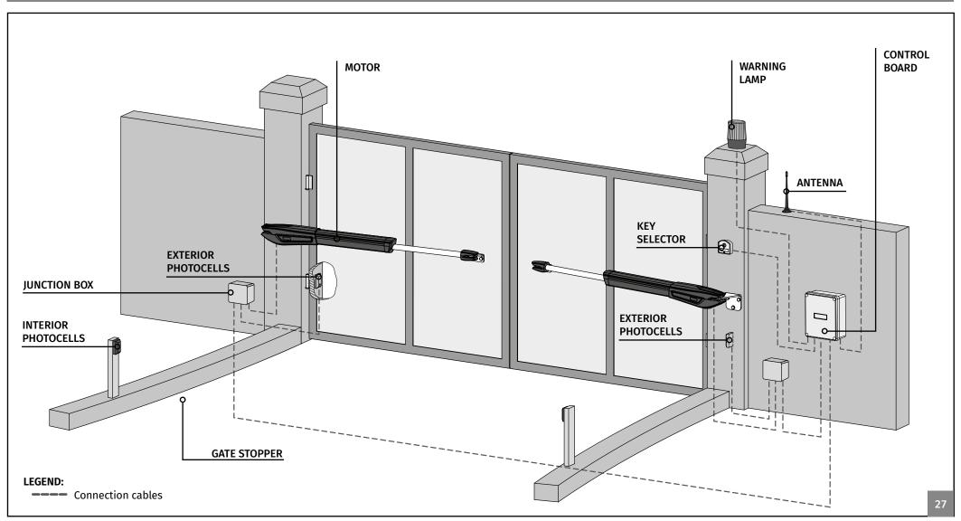
It is important to use mechanical stoppers in the opening and closing position of the gate. If not respected, components of the automation may suffer efforts for which they were not prepared, and as a result will be damaged.
