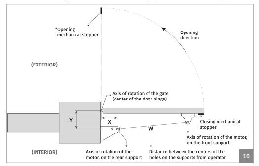
On the Illustrated diagrams below and on the next page, are the **dimensions for the installation** of the automated system.
