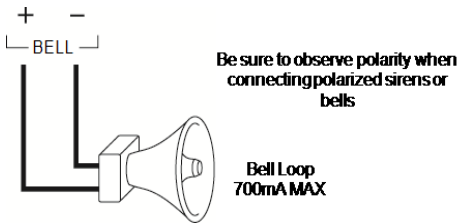
Figure 2-13 Bell Wiring
