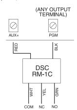
PGM1 can sink up to 50mA of current. Connect the positive side of the LED or buzzer to AUX+, the negative side to PGM1. PGM2 operates similarly to PGM1. If more than 50 mA of current are required, a relay must be used.
