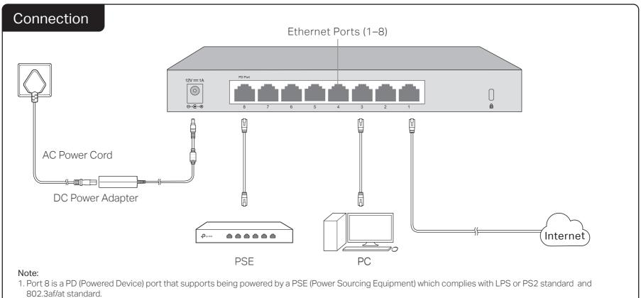
2. The DC power input takes precedence over the PD port. If the DC input fails, the PoE input on the PD port will supply power instead.
