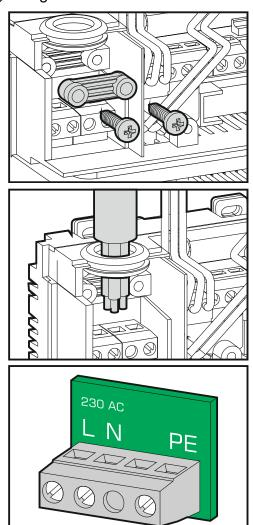
11. Screw the wire fastening element.
