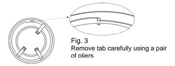
The sounder can then only be removed by using a special Removal Tool (TSC-SRT), which is available from Hochiki Europe (UK) Ltd.
