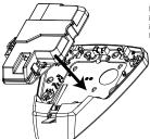
NOTE: The bottom battery holder should be installed as shown -in order to allow to installation or removal of the Deltabell Module
