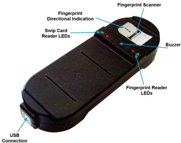
Figure 2: CP-R25 Components
