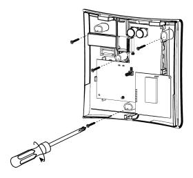
Figure: 2 Mounting the HSM2HOST
