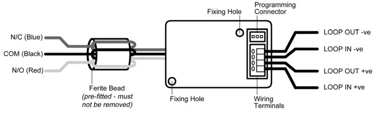
Fig 1 CHQ-SOM Wiring
