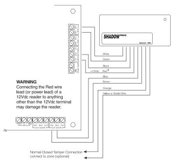
**NOTE**: Only use the +12V power supply when using ShadowProx Readers.
