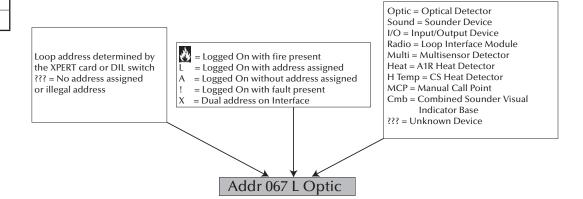
Note: Combined sounder visual indicator base shows two addresses, first address in the detector followed by the sounder visual indicator as shown below.
