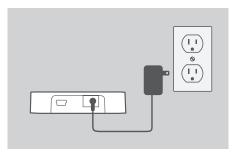
1. Plug the power adapter into the connector located on the back of the DUB-H4. Plug the other end into a wall outlet. The LED on the DUB-H4 will turn green to indicate that the hub is receiving power.
