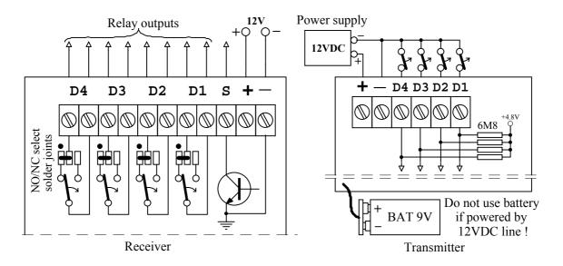
Unused transmitter inputs must be connected to receiver's ground (-V). When receiver is powered by 12VDC line remove battery otherwise the battery may be damaged.
