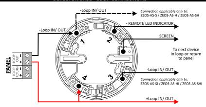
NOTE: Positive terminal of remote indicator should be connected to terminal 4 (+ Loop IN/OUT)
