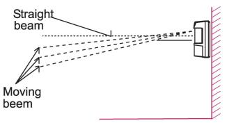
Changing the detection range is achieved by sliding the upper detection element up or down.
