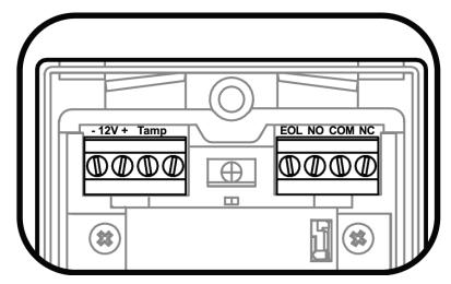
Terminal 1 - Marked "-" (GND) - Connect to the ground of the CP.
