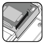
Slide the detection element down for long range or up for short range detection.
