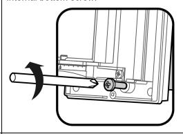
8. Attach the rear bracket to the wall or a pole using mounting screws or metal bands.
