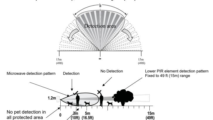
Upper PIR element detection pattern Adjustable between 10 ft to 49 ft (3m to 15m)
