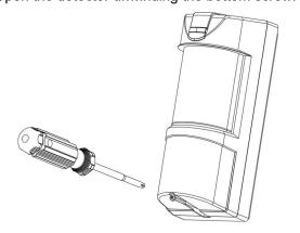
7. Release the detector body from the metal bracket by polling front and up.
