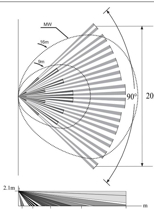
Note: TITAN MW AM complies with GRADE 3 when the installation height is <2.0 m and has coverage range detection from 0.5m to 15m.
