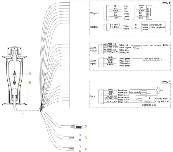
Figure 2-1 Cable connection
