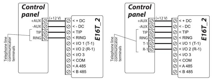
Communicator wiring diagram, when telephone line supervision is not set.
