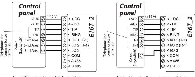
Arming/Disarming the panel via keyswitch zone, when telephone line supervision is not set.
