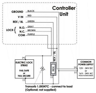
Figure 3: Wiring Diagram for Lock Strike Relay & REX
