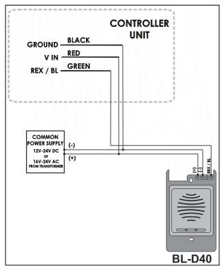
Figure 5: Wiring Diagram for the BL-D40 External Sounder
