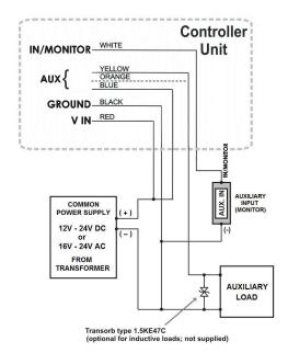
Figure 4: Wiring Diagram for Auxiliary Input & Output
