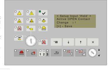
Use the buttons  $\stackrel{\downarrow}{}$  (Down) and  $\stackrel{\uparrow}{}$  (Up) to change alternatively the parameter, the button  $\stackrel{\downarrow}{}$  to confirm the new value and the button  $\stackrel{\times}{}$  to exit.
