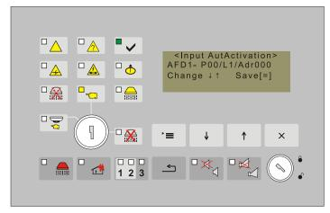
13.4.2.6.3. Inputs "Mode Manual/Automatic", "Disable Extinguishing" and "Hold Extinguishing" are to be set by the same procedure.
