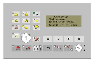
13.4.2.3. Set Up speed on CAN network communication.
