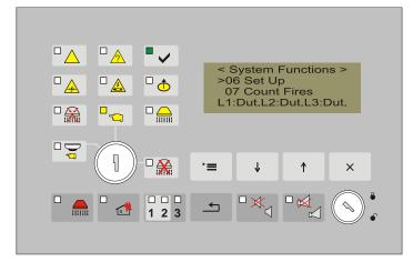
Enter a password (four-digit number) to have an access to the menu. The factory set password is "0000".
