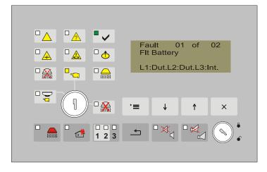
**Example:** Two fault conditions are registered: fault in the back up battery power supply and interruption of line 3. The common indicator for fault condition and the specific indicator for power supply fault are illuminated.
