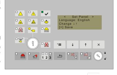
When the parameter is changed and the new value is saved with the button  $\stackrel{:}{\sqsubseteq}$  a text message "Saved!" appears! Exit – [x]". The fire extinguishing control panel is factory set to English language.
