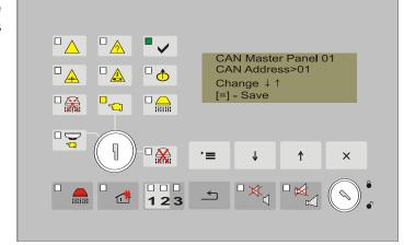
In articles 02÷08 from the Menu, insert by analogical order the addresses of the other control panels series 7000, comminicating with the Extinguishing Panel.
