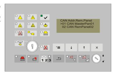
In article 1 of the subordinate menu enter the address of the "Master" panel. The panel is required to be from series 7000.
