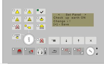
Use the buttons  $\downarrow$  (Down) and  $\uparrow$  (Up) to change alternatively the parameter, the button  $\stackrel{*}{\sqsubseteq}$  to confirm the new value and the button  $\stackrel{\times}{\sqsubseteq}$  to exit.
