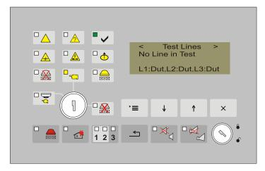
If there is/are line/lines in test, their numbers appear on the display. Information on the changed status is provided on the fourth line of the display.
