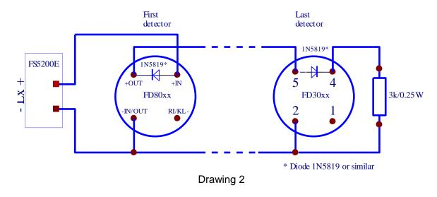
Use automatic fire detectors FD3000 or FD8000 series or other compatible automatic fire detectors. Mount resistor 3 k $\Omega$  / 0.25W on the last fire detector in the line.
