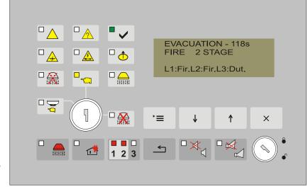
Text message for the phase of fire alarm, the remaining time for activation of the extinguishing devices and the current status of the lines is visualized on the display. The local sounder produces continuous signal. Potential free relays Rele 2St and Rele Fire are activated. Voltage 28V DC is supplied to the sounder output S2.
