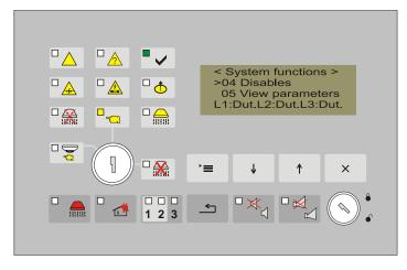
When the function to disable a fire alarm line or an output from the fire extinguishing control panel is selected from the subordinate menu, a screen appears displaying the current status of the disable in the specific
