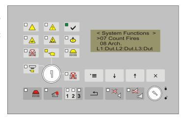
The screen provides information about the entries of the number of times when the fire extinguishing control panel has entered Fire condition.
