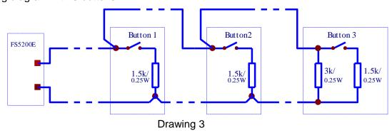
When the contact is closed the fire extinguishing control panel accepts the button to be active.
