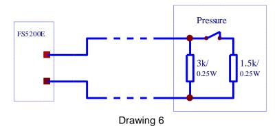
Set up the input active status: OPEN or CLOSED contact from menu System functions > Set up > Input/Outputs > Low Press input.
