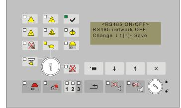
13.4.1.3. The fire extinguishing control panel supports menus and screens in two of three languages:
