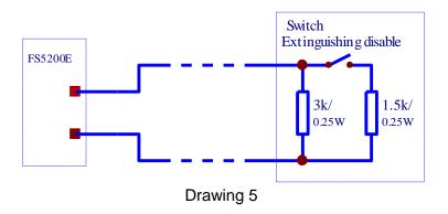
When the contact is closed the fire extinguishing control panel accepts Disable Extinguishing. Output Open collector type is activated in Disable Extinguishing. That output could be used as switch indication, if this option is provided.
