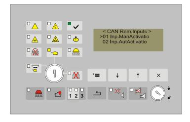
13.4.2.6.1. Input Manual Activation includes the opportunity for activation from manual call point type FD7150, of system series 7000, operating in a common network together with Fire Extinguishing Control Panel. Insert data for the address of the Control Panel, the address of the loop and the address of the manual call point. The admissible number of manual call points that can be included is 5.
