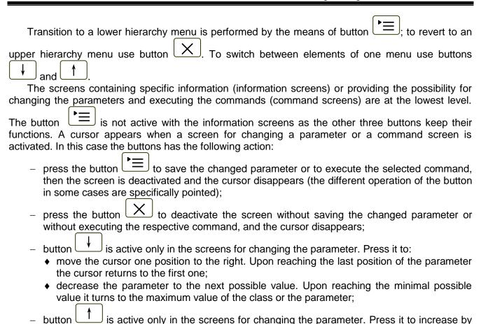
one unit the class marked by the cursor or to increase the parameter to its next possible value. In both cases upon reaching the maximum possible value it turns to the minimum value of the
