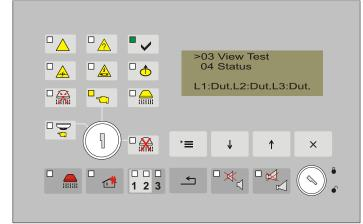
Press the button to display the screen to view the lines in test.
