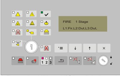
Potential free relays Rele 1St and Rele Fire are activated. Voltage 28V DC is supplied to the sounder output S1.
