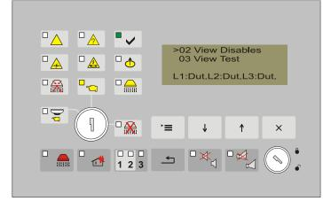
Press the button  $\stackrel{\triangleright}{\equiv}$  to visualize the screen to view the entered disables.
