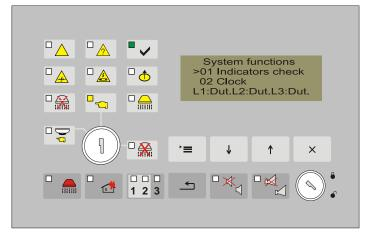
Press the button . All LEDs indicators are illuminated and the sounder produces continuous signal.
