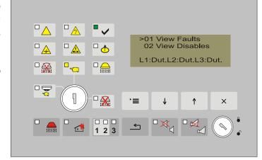
If there are no faults a text message "No Faults" appears on the display.
