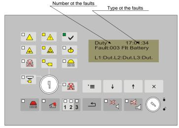
Upon non-fatal faults when the fire extinguishing control panel is not in Fire condition, the following information screens appear:
