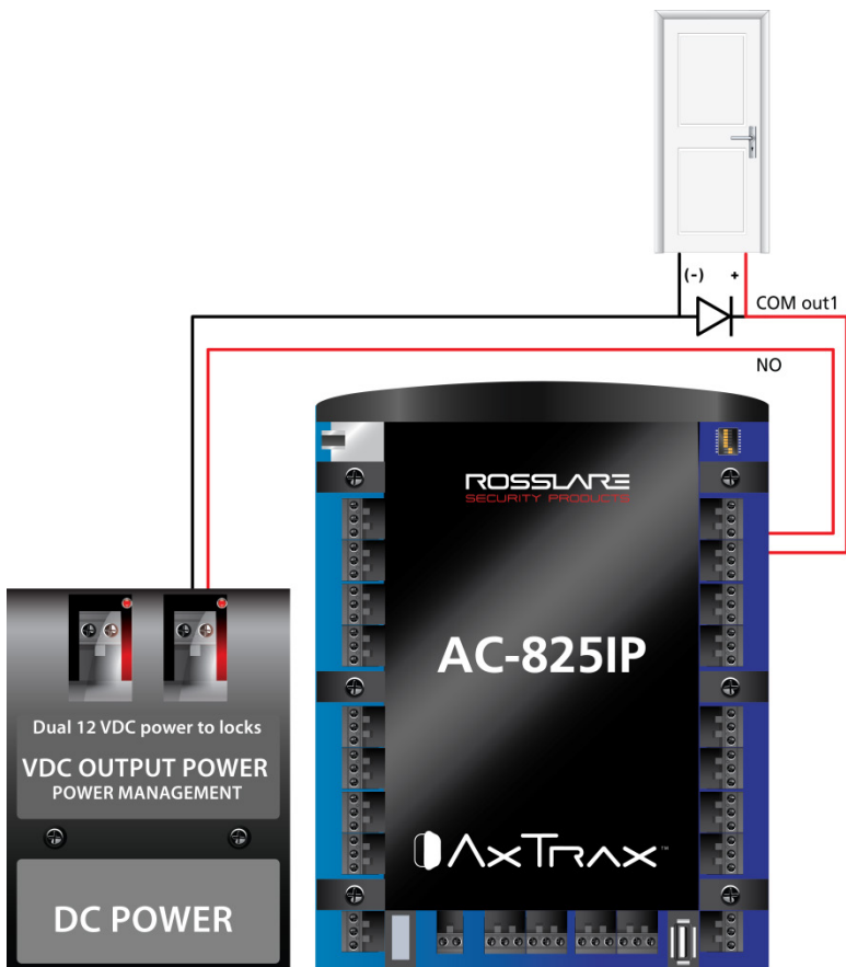
Figure 3: Door Lock – Failed Close
