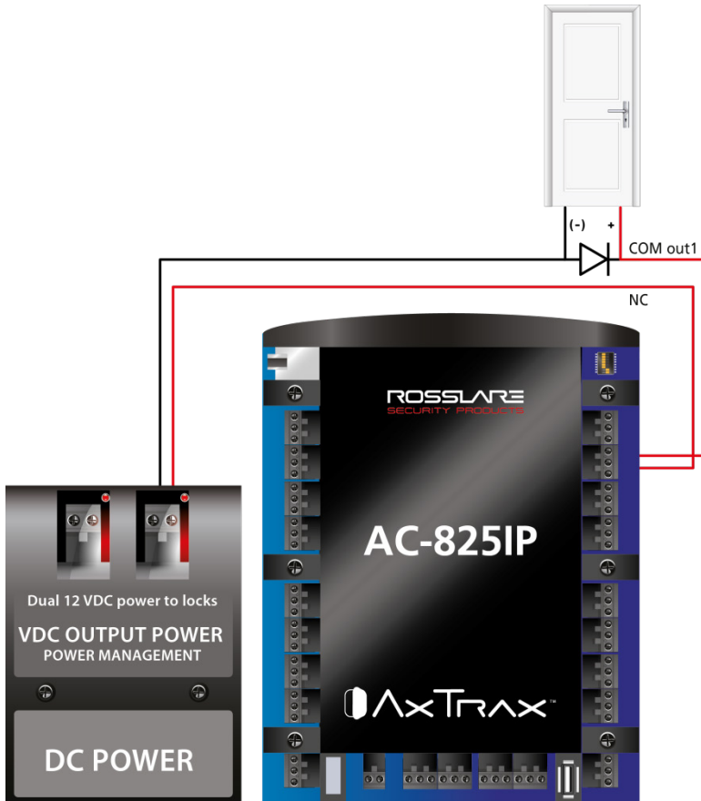
Figure 4: Door Lock – Failed Open
