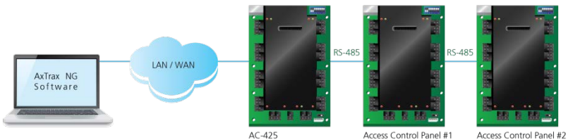
Figure 21: Connecting Multiple Access control panels with AC-425
