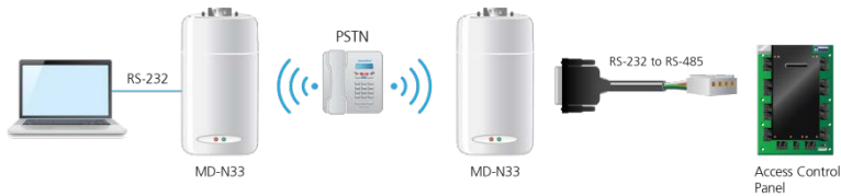
Figure 22: Remote Site Modem Configuration
