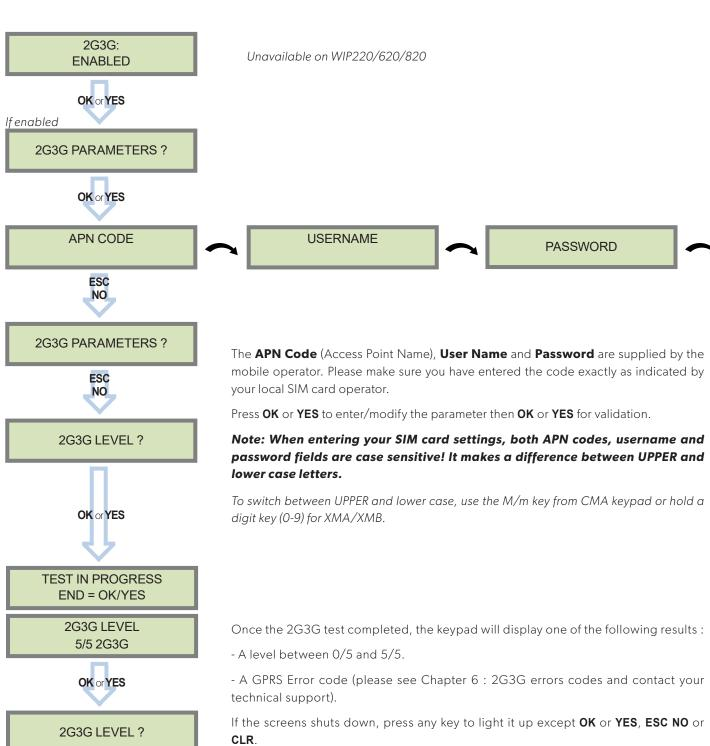
The 2G3G level test can last several minutes. Do not interrupt the test or remove the SIM card during the test.
