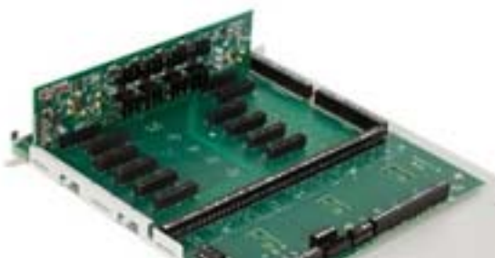
Figure 2-3 Secure Position for Circuit Boards in the Backplane
