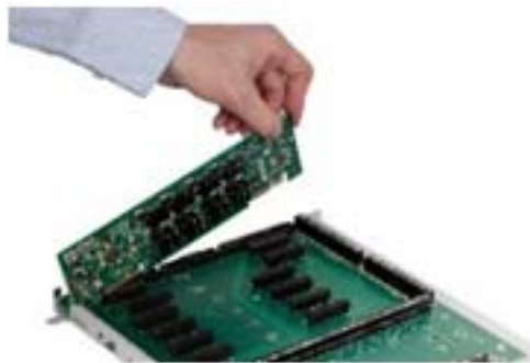
Figure 2-3 Secure Position for Circuit Boards in the Backplane
