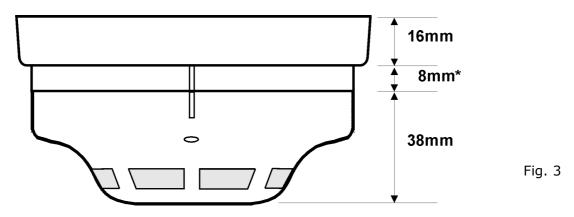
\*Shown with the YBN style of Base at 8mm, other bases such as the YBO style are deeper.
