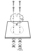
Secure the mounting bracket to the ceiling tile using four M3x30 pan-head screws, washers, and wing nuts, as shown on the left.
