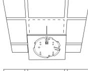
Feed the Ethernet cable through the hole and set the ceiling tile back into place.
