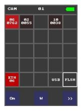
To search and localize the detected video camera press the cell and hold for two seconds, then a scale (column) with the signal level will appear on the screen.
