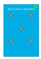
Calibration is performed by pressing the sharp end of the stylus (supplied in the delivery set) into the centers of the "crosshair" of the circles appearing on the screen.
