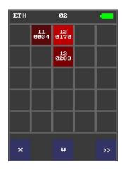
The detected signals emitted from devices, which are using Ethernet protocol (IP cameras, computers, Wi-Fi routers, switches and other peripheral devices) are grouped in the "ETH" cell (the cell is colored in red).
