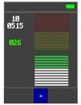
Press and hold the selected table cell for two seconds with your finger or stylus, and a multi-colored scale (column) with the signal level will appear on the screen. To the left of the scale, information about the signal is displayed.
