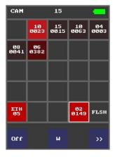
For searching and localizing the detected video camera press the cell and hold for two seconds, then a scale (column) with the signal level will appear on the screen.
