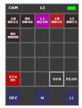
To enable or disable the mode of detecting USB cameras, briefly press the stylus or your finger on the "USB" cell, the "On" or "Off" checkbox will appear in the lower left corner of the screen.
