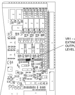
VR1 – ADJUST EXTINGUISHANT OUTPUT MONITORING
