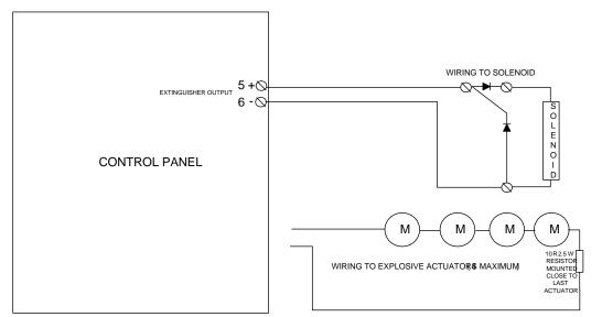
To enable monitoring of devices such as Metron actuators which have a very low resistance, the short circuit threshold level needs to be adjusted to suit. To do this, first remove the cover from the K6002 PCB mounted on the back chassis by removing the single screw that hold the cover in place and put the screw and cover aside.
