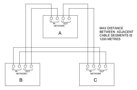
Network boards are fitted with isolators, which disconnect faulty sections of cable and allow the network to continue working by using the return path so it is most important that this wiring configuration be adhered to.
