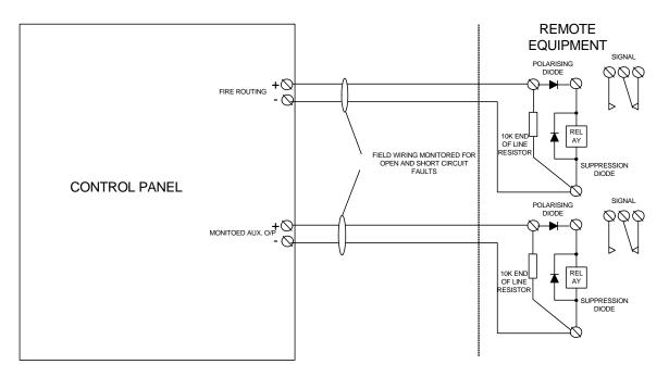
Connections to the remote equipment should be as shown above. It is important if the device at the receiving end is an electromagnetic device such as a relay that polarising and suppression diodes are fitted to prevent operation of the device in the normal condition and to suppress any interference generated by the device when it operates.
