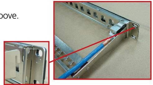
C.) Insert the Jack into the opening in the Patchpanel at an angle with the non-flexing side of the keystone latch facing down. See foto 3.
