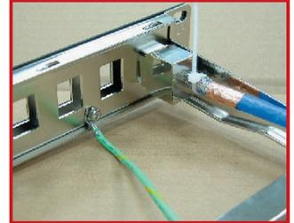
B.) Align the tongue on the other side of the wire minder with the corresponding groove on the Patchpanel and insert it into the groove. Push the wire minder down in the slot. See foto 2
