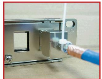
E.) After the installation of a Jack, use a tie wrap to attach their wires to the cable management as shown in foto 5. Do not overtighten the tie wrap! It should be snug, but not so tight that it crushes the wires.
