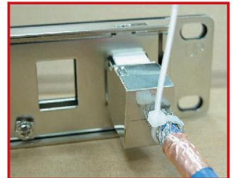
D.) With the bottom latch engaged to the Patchpanel, rotate the Jack upward until the flexing side of the keystone latch engages with the Patchpanel as shown in foto 4. There should be a slight clicking sound as the latch engages.
