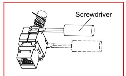
In order to remove the connector clip, insert a small screwdriver into the slot.
