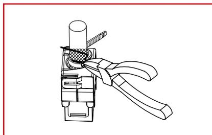
Cut the tie wrap as close to the cable as possible. Do not cut the drain wire or damage.
