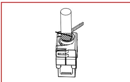
Tie-wrap the drain wire to the shield. Do not over tighten the tie wrap! If should be snug, but not so tight that it crushes the wires. If necessary cut the excess shield without damage to the cable jacket.
