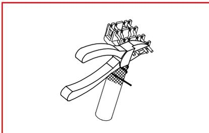
Cut the excess wire off as close to the edge of the cap as possible.
