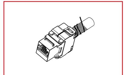
Ensure that the drain wire is wrapped around the cable and shield.
