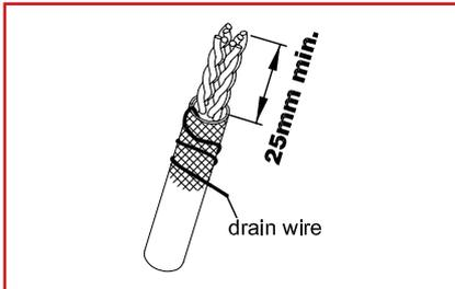
Strip a minimum of 25 mm of jacket from the end of cable, pull the foil or braided shield back over the jacket as shown and wrap the drain wire around the shield.
