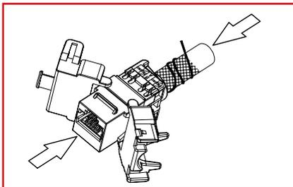
Align the cap with the IDC towers and press it into position.
