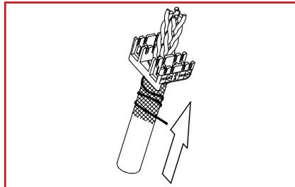
Insert the wires from the stripped cable into the cap through the hole as shown.
