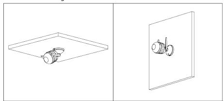
Figure 4-3 Installation methods
