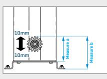
The pinion can rise or fall 10mm from the standard position (on the left). Standard height of the pinion upper limit
