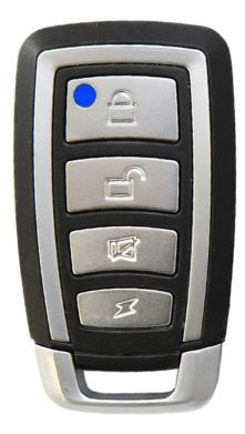
dynamic code system KEELOQ® of Microchip Corp. USA • operating frequency: 433,92 MHz • average range: 100m in open field • power supply: alkaline battery 2x CR2016 • number of channels: 4 • external dimmensions: 55/31/13
