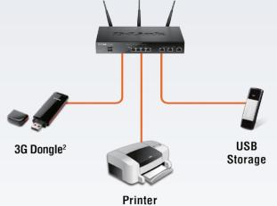
Supports one (DSR-250N) or two (DSR-1000AC) USB 2.0 devices to extend functionality.
