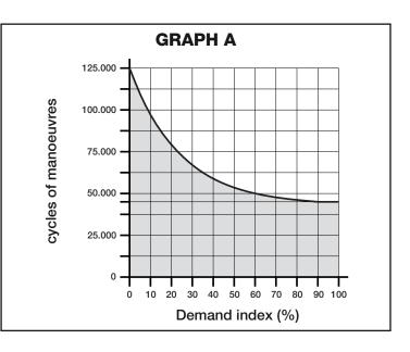
Example of calculation of durability of a Wingo WG5024 gear motor (refer to Table 2 and Graph A):
