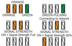
SIGNAL STRENGTH OFF = No Signal Strength
