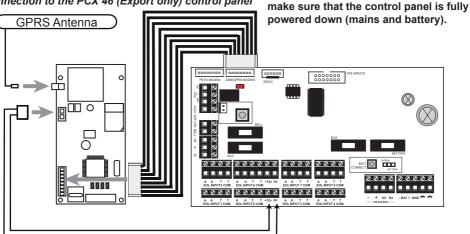
NOTE: When connecting a Digi GPRS to the Enforcer control panel, please use the power connector marked 'GSM modem' on the inside of the plastics.
