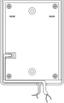
4. If there is no hole on the wall, you can allocate the wire on the groove around the case as appeared in the figure.
