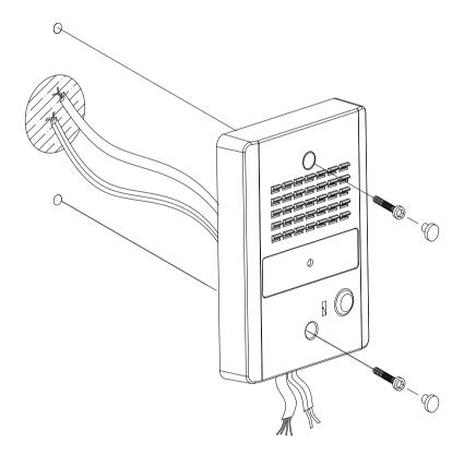
5. Place the system on the wall and mount with screws supplied.
