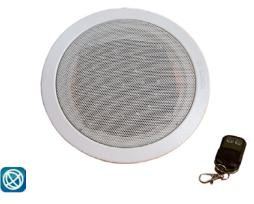
An array of 24 ultrasonic transducers in the SEL-324A "Speaker" are installed in a thin (the height of the device is 40 mm) drum-shaped ceiling speaker case, providing easy deployment into ceiling speaker mounting points, that are commonly available in rooms as mounts for emergency speaker audio systems.
