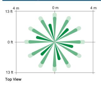
Broad Coverage: Up to 7.5 m x 360° (24 ft x 360°). Provides 360° coverage pattern. Coverage diameter is approximately two times the mounting height.
