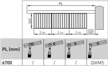
WARNING: for PL>4000 mm, you must use the fixed support QIKAF-QIKAFE or the mobile support QIKAM. With the fixed support with the electromagnetic block QIKAFE installed, use the configurations indicated for the mobile support QIKAM.
