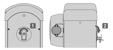
In the event of a fault or power failure, insert the key, turn it anticlockwise and completely open the hatch. Manually open the barrier.
