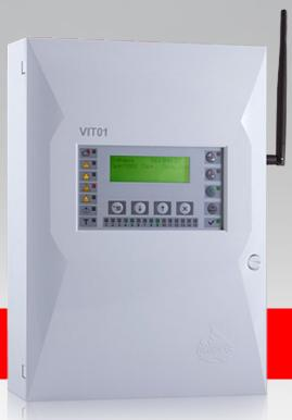
In case of fire event, the results of the combustion are detected from the wireless point fire detector and through radio frequency channel a fire status message is sent to the VIT01 fire control panel. The system components installed at the site are organized into a radio network. The maximum number of independent wireless systems at one premise is 16.
