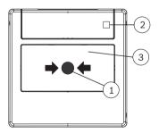
Pressing the black marking (1) breaks the glass pane (3), which triggers the alarm and causes the LED (2) to flash.
