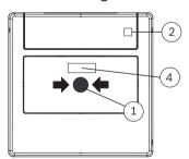
Pressing the black marking (1) triggers the alarm. The alarm status is indicated by the changed window color (4) and the flashing LED (2).
