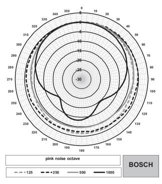
Polar diagram horizontal (low frequency). Normalized at 0 degrees axis.
